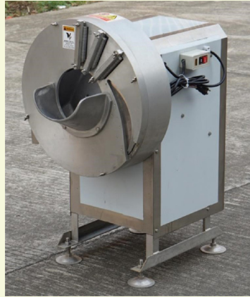
Gambar 8. Mesin perajang pisang (Sumber gambar: https://id.aliexpress.com )
